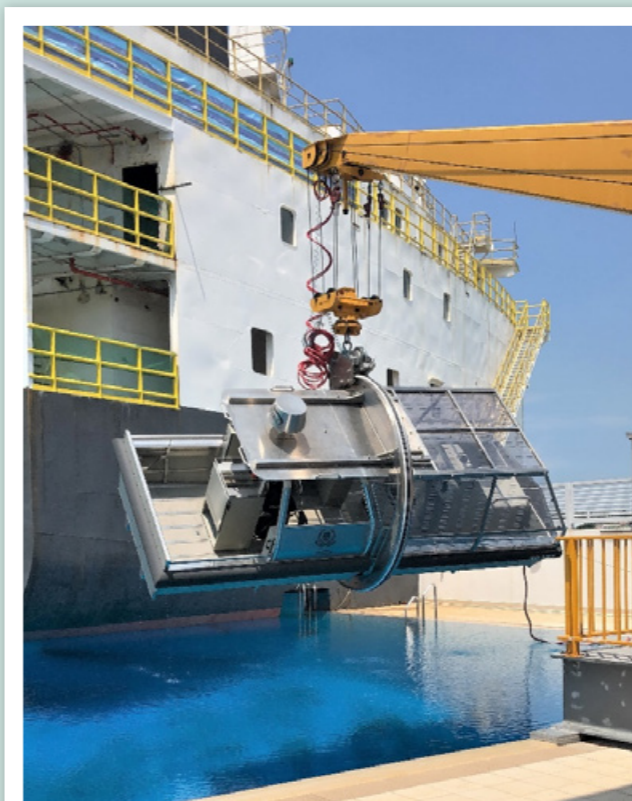
The UETS automatic rig lifting the boat structure after undergoing a capsize simulation.
