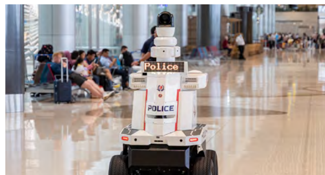
The patrol robot is equipped with features including speakers, siren, blinkers, a display panel and a two-way communication function.
