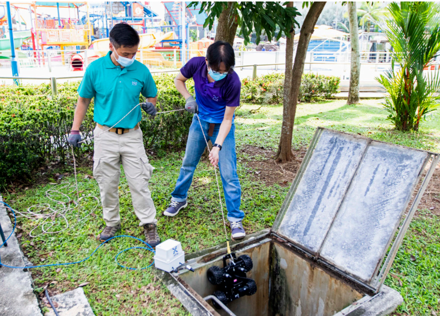
SecCom and HTX officers demonstrating how the MiniX is deployed into a sewage drain.
