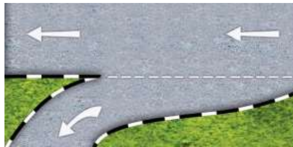
(i) Broken White Line at Decelerating Lane
