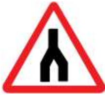
Dual-carriageway ends (Slow down. Keep left. Beware of oncoming traffic)
