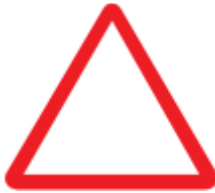
Vehicle breakdown sign (To be placed at least 20 metres from the rear of the vehicle)
