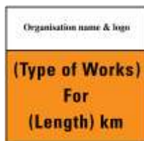
Start of Work Zone
