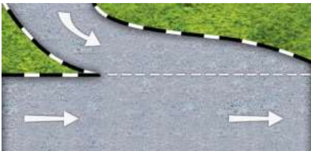
(h) Broken White Line at Accelerating Lane
