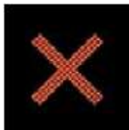
The RED Cross indicates that the lane is closed to traffic
