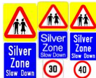
Start of silver zone (Slow down and look out for elderly pedestrians crossing the road ahead. Vehicles shall not travel above the posted speed limit as indicated in the speed limit sign attached)
