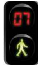
Countdown timer (Indicates the remaining time (in seconds) for pedestrians to cross the road)
