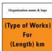
Start of Work Zone
