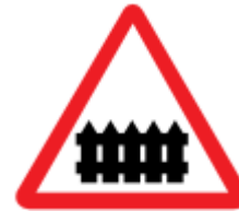
Gated level crossing (Slow down. Beware of gate closing)
