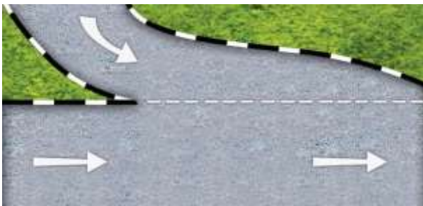
(h) Broken White Line at Accelerating Lane
