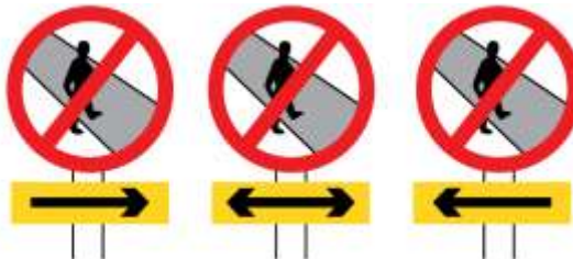
Pedestrian crossing Prohibition (Within these signs, pedestrians must use the designated crossing when crossing the road)
