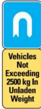
U-turn sign with vehicle weight restriction (U-turn ahead for vehicles not exceeding the weight limit as stated on the sign)
