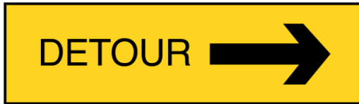
Detour in the direction indicated
