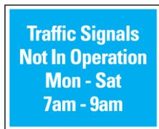
Traffic signals operating hours (Traffic signals not in operation during stated hours)
