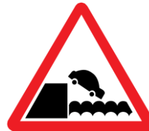
Road leading to quay, river bank or sea (Slow down. Beware of road ending ahead)
