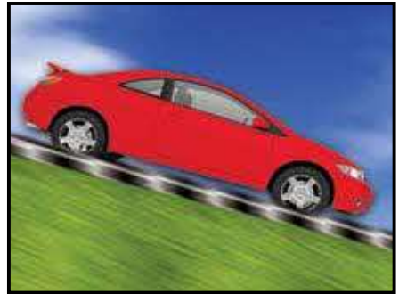
(b) On a steep downhill slope, use the second or the first gear.
