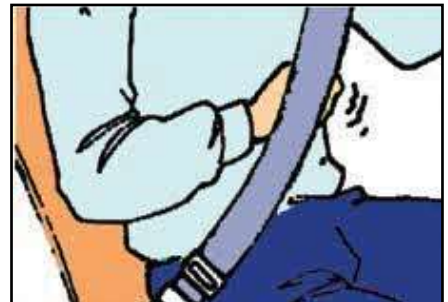
(f) For the non-retractable type of seat belt, the slack should not be more than a clenched fist space between the shoulder belt and your chest.
