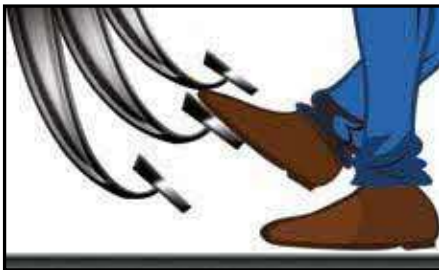
(a) You should use the ball of your right foot to depress the brake pedal.
