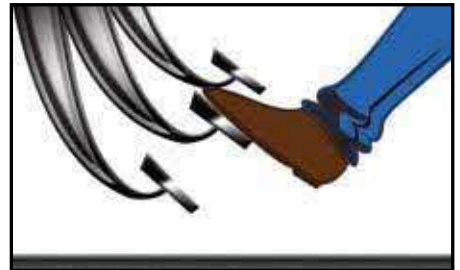
(b) Your heel should not touch the floorboard when the brake pedal is being used.
