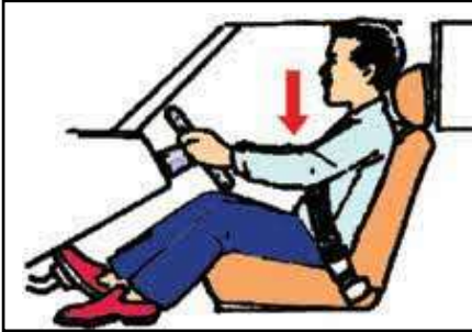
(a) Sit upright and lean against the backrest with both hands comfortably holding the steering wheel. Arms should be slightly bent.
