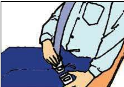
(e) Fasten the seat belt only after you have adjusted the seat and are in the correct driving posture.
