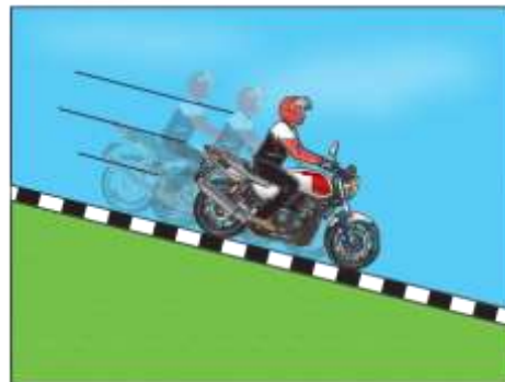
(b) On a steep downhill slope, use the 2nd or the 1st gear.
