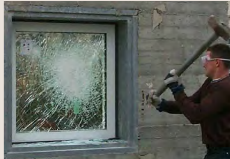
Figure 37: Testing of 15 minutes forced entry resistant window
