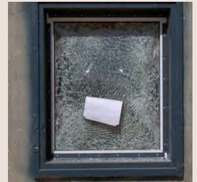
Figure 31: A window protected by mechanically anchored ASF for basic blast level (after explosion)
