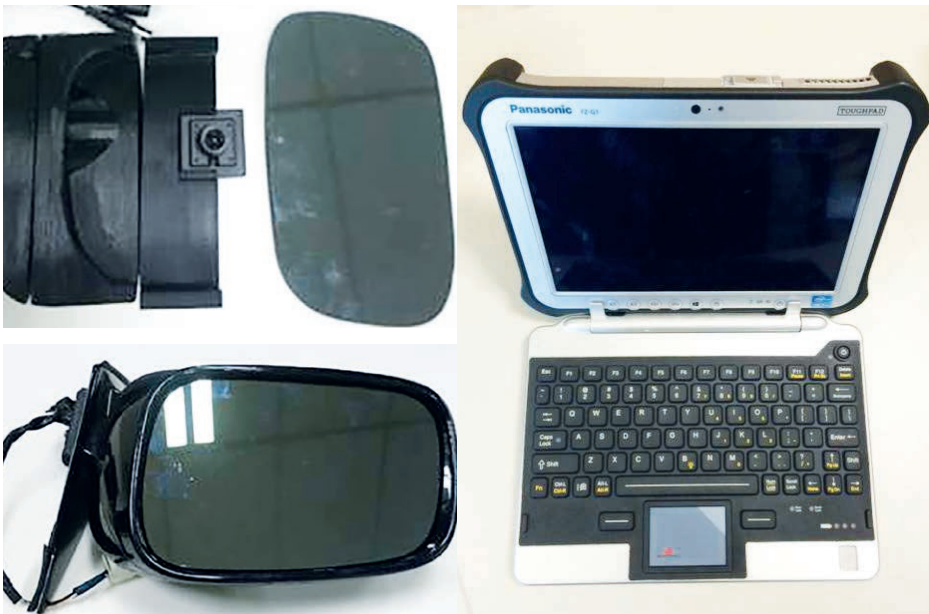
Camera is concealed in the side mirror of a motorised vehicle to videotape acts of vandalism on the vehicle
